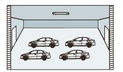
With sufficient ambient light, the light will not be switched on even if with motion signal.
