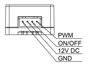
\*The sensor is designed to connect one load only. Connect more than one load may damage the sensor.
