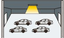
When motion is detected, the sensor will switch on the light to 100% brighteness
