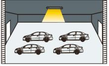
With insufficient ambient light, the sensor switches on the light when motion is detected.
