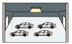
If there is no motion detected, the light will be remained at a low light level all the time.
